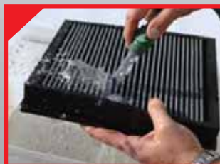
Rinse thoroughly and repeat cleaning process until filter rinses clear
